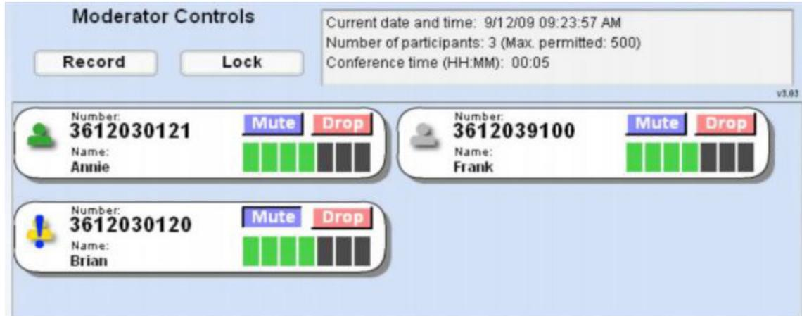
The panel at the top right provides information about the current conference. To the left of this are two buttons to control recording and locking the conference, which are described later in this section. Each participant in the conference is represented by a panel with a telephone number at the top.
